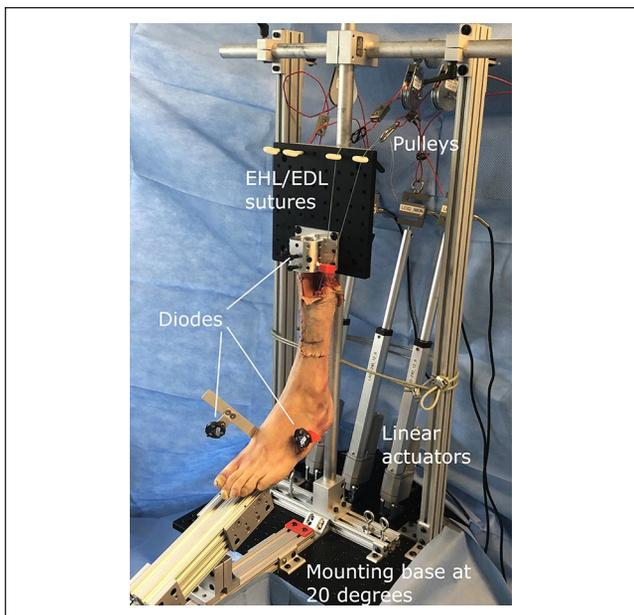
**Figure 2.** Specimen mounted into the custom testing apparatus with infrared diodes mounted to the first and fifth metatarsals and extensor tendon suture loops attached to the linear actuators via a pulley system. Oblique lateral view with labeled experimental components. EDL, extensor digitorum longus; EHL, extensor hallucis longus.
