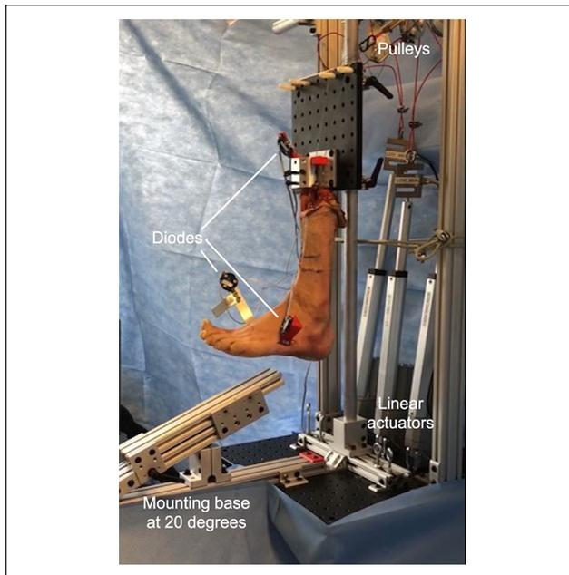
**Figure 4.** Intact state testing of extensor hallucis longus and extensor digitorum longus tendons with labeled components. Metatarsophalangeal hyperextension seen during intact state testing that mimics clinical claw toe pathology.
