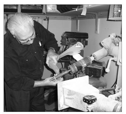
FIGURE 1: Frank Gramaglia, of Hanger Prosthetics and Orthotics in Havertown, PA, trims the front of the brace and then grinds the edge smooth.
